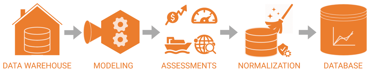
Figure 4.1 Modeling flow: warehouse data is modeled into assessments, normalized to a common basis, and stored in the published database.
